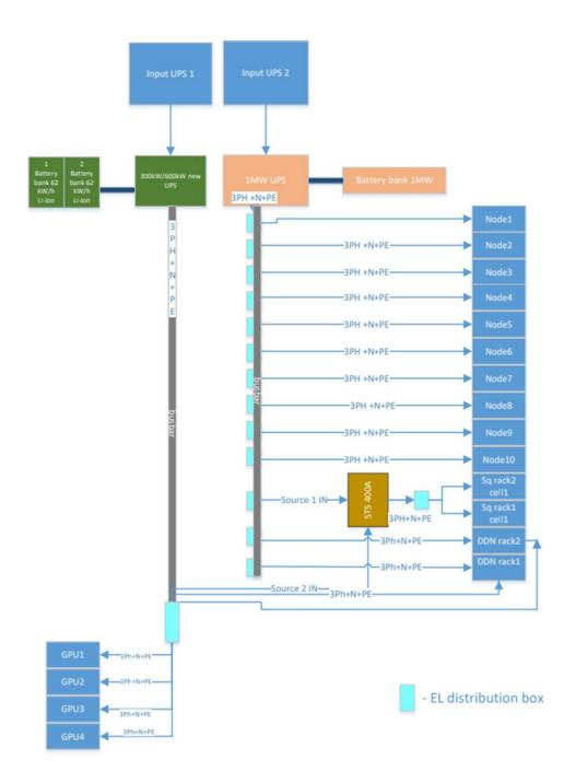
Technical requirements for the new modular 3-phase UPS, 300kW (250kW+50kW), N+1, hot-swap, extendable to 600kW.
