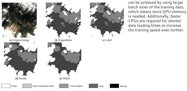
Comparison of L2A prediction output for a 512 × 512 pixels sub-tile in the test dataset. (a) Original Sentinel-2 True-Color Image; (b) KappaMask classification map; (c) Segmentation mask prepared by a human labeller; (d) Fmask classification map; (e) MAJA classification map.
