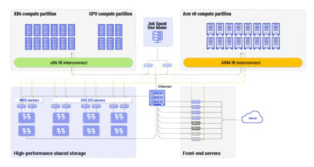
Figure 5: The Deucalion supercomputer architecture
