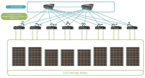
**of usable Ceph storage** (with 16+3 erasure coded pools). Internal Ceph Network contains 8 Mellanox SN2010 switches, each 18x 25GbE + 4x 100GbE ports.
