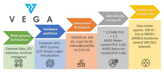
Figure 9 - The Vega system in a glance
