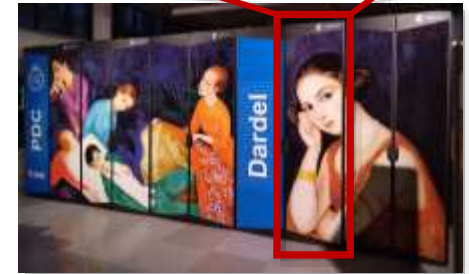
Dardel: 56 nodes, 448 MI250X GCDs, ≈10 PFlop/s
